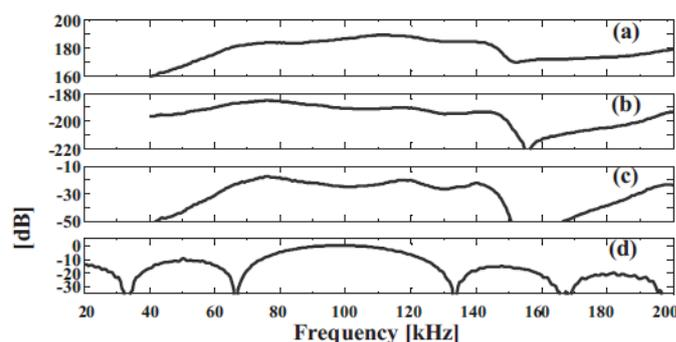
FIG.1 Frequency response of (a) transmitting and (b) receiving sound by the custom made transducer. Product of both sensitivity (c) still keeps the broadband capability comparing with the main lobe of the three waves sinusoidal tone burst (d)
