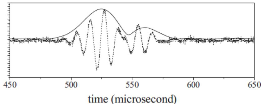
FIG.4 Envelope extraction of the echo was conducted by cross correlation between incident and
