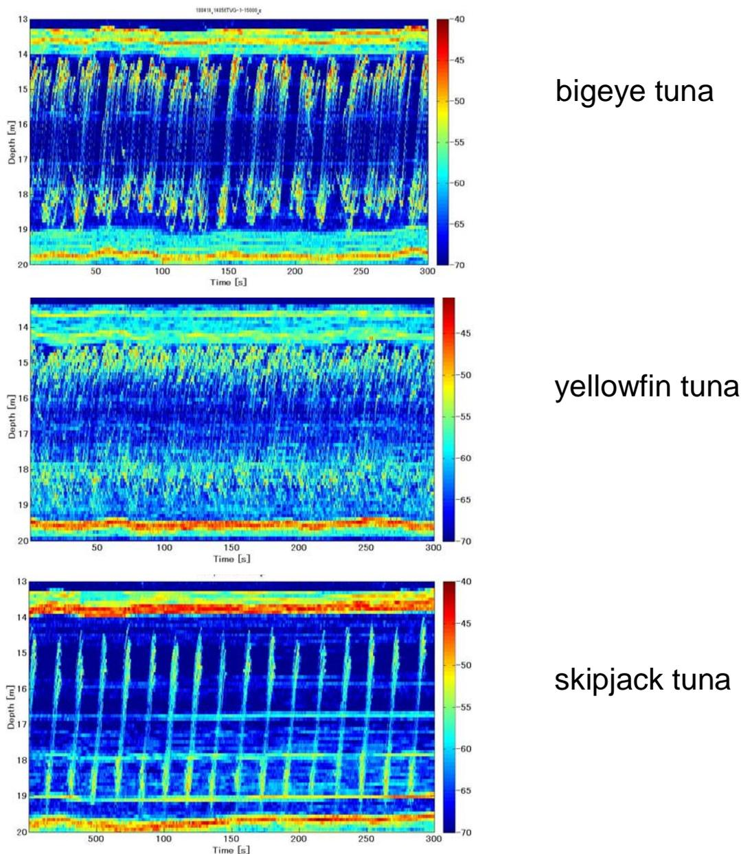
FIG.5 Echogram of bigeye tuna, yellowfin tuna, and skipjack tuna Each trace corresponds to individual fish except for skipjack tuna. Skipjack tuna swam in a group, which echogram showed a
