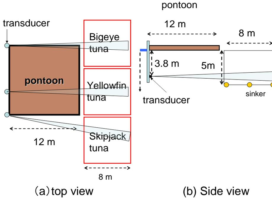
FIG.3 Three net pens were fixed right next each other beside the pontoon. Each pen had single species of fish bigeye tuna, yellowfin tuna and skipjack tuna. They swam in circle and the acoustic beam was projected horizontally from the transducer as shown in blue long triangles. The position of the transducer was adjusted to point the beam to the center of each enclosure except for skipjack tuna. Because of the location of the skipjack pen, the acoustic beam axis was at an angle.
