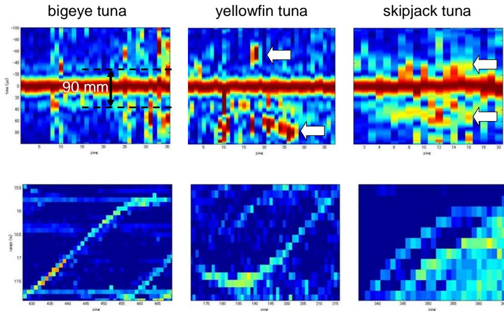
FIG. 6 Envelope (top) and echogram (bottom) patterns of three tuna species. Red center line of the envelope pattern indicate the swim bladder or spine, which are the major reflectors at the center of the fish body. There are two side robes above and below of the center. These side robes seemed to come from the both sides surface of the fish body. Intensity of the side robes were stronger for a yellowfin tuna and a skipjack tuna than that of a bigeye tuna.
