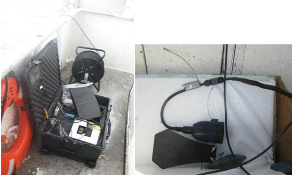
**Figure 1. Splashcam video system with topside viewing and recording gear (left) and drop camera equipped with archival tag for depth measurement**
