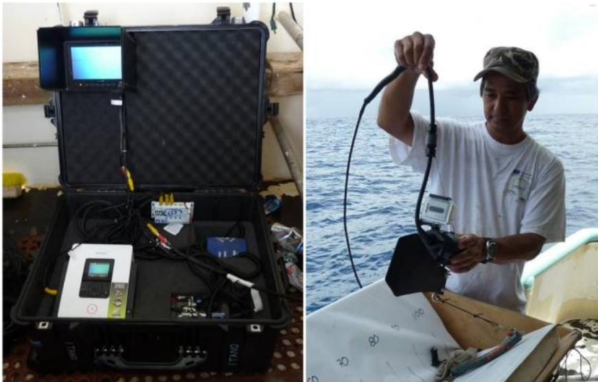
**Figure 4. Splashcam viewing and recording system (left) and GoPro high definition video camera mounted on the Splashcam camera head prior to deployment.**
