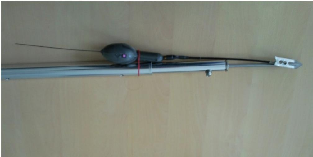
**Figure 1.** Configuration of tag ready for deployment in the Escalle et al. (2014) study showing 4-meter tagging pole, applicator pin, titanium anchor, 20 cm tag tether, and miniPAT tag with rubber band.
