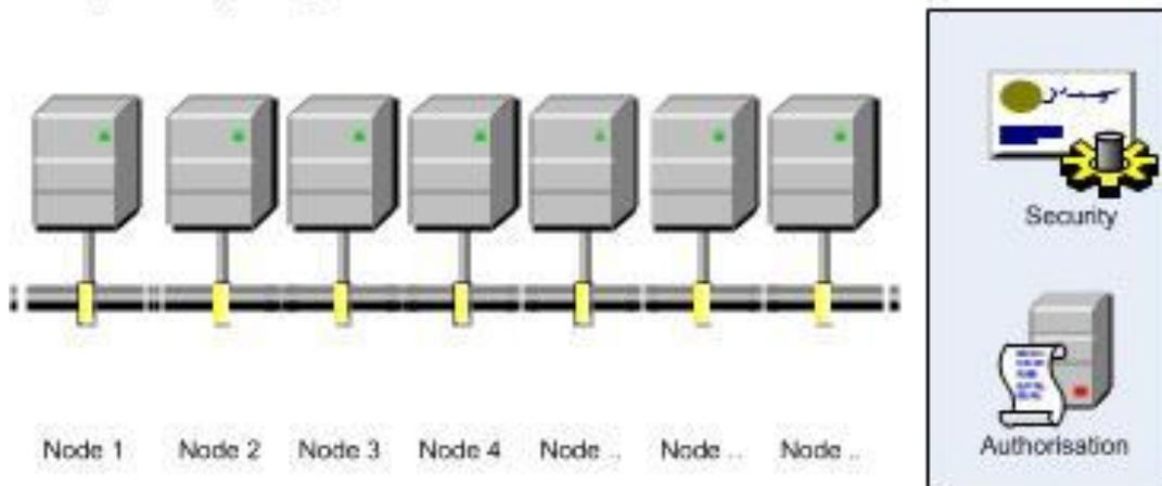
No matter how the physical topology is made, the software can be configured so that it appears that every node is directly communicating with any other node.
