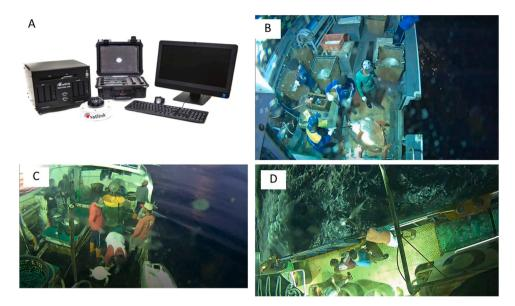
Fig. 1. The Satlink Seatube Lite EM System (A); example images of the EM system: Working deck camera, showing catch of opah (B); working deck camera showing catch of marine turtle (C); and catch of a yellowfin tuna (D).
