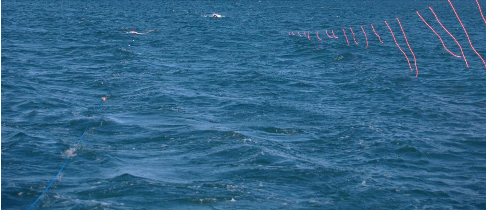
Figure 7. Tori line 8 showing the large road cone comprising the in-water section and the splash it created at 4 knots. The rope used to measure aerial extent (marked with floats at 5-m intervals) is visible on the left.
