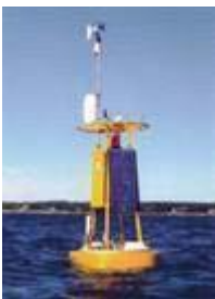
EMM2000 Coastal Monitoring Buoy
