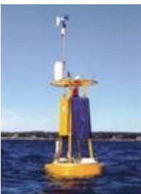
EMM2000 Coastal Monitoring Buoy
