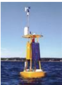
EMM2000 Coastal Monitoring Buoy
