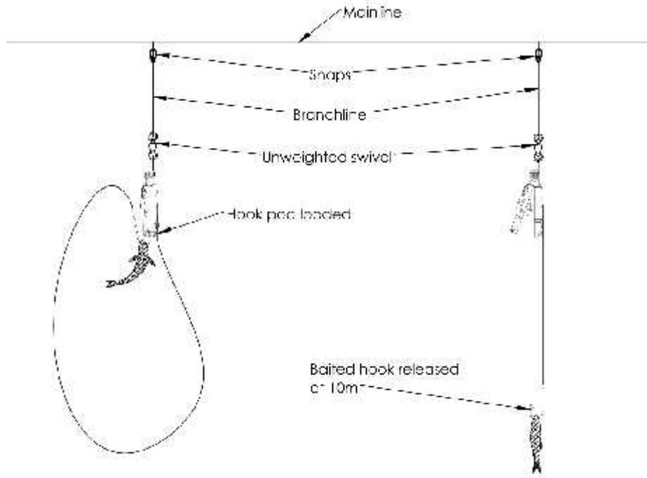
Figure 2. The Hook Pod *in situ* prior to and after the pressure release mechanism opens the pod
