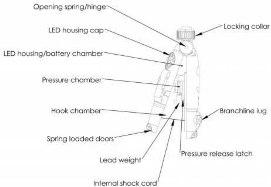
Figure 1. Components of the Hook Pod
