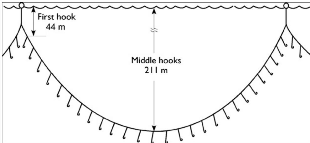
**Figure 1.** Diagram of a typical pelagic longline configuration showing hooks attached to the mainline by branchlines and suspended between floats. Note that depths shown are average depths from Hawaii-based tuna longline fishery and the length of the branch lines and the average distance between branchlines are not to scale. (Source: Beverly et al. 2009).
