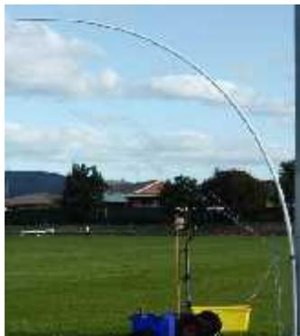
Figure 2. A tori pole under 20 kg of drag - more than was ever required to achieve an aerial extent of 80 m during the on-land trials.
