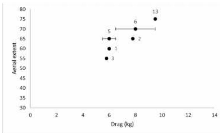
Figure 8. Drag and aerial extent delivered by the tori line designs tested at 6 knots on vessel A. Error bars show ranges in drag or aerial extent where the in-water section did not deliver consistent drag. Numbers adjacent to points refer to the construction of the in-water section (Table 4). The aerial section of all tori lines comprised 70 m of 3-mm diameter Dyneema with single 9-mm Kraton streamers placed at 2.5 m intervals.
