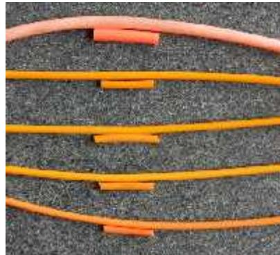
Figure 5. Five streamer materials after seven months exposure to ambient exterior conditions. The small segments are the same materials pre-exposure. The 9-mm diameter Kraton-like material is at the top, and T061 – T064 are in order from the second to top to the bottom of the figure.
