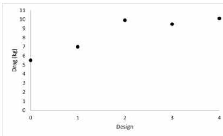
Figure 4. Drag required to provide 70 m aerial extent for a tori line with a 3 mm Dyneema backbone deployed at 7 m high, with different combinations of streamers and shark clips attached. Design 0: streamers at 5 m intervals; 1: streamers at 5 m intervals and 10 shark clips attached; 2: streamers at 2.5 m intervals with no shark clips; 3: streamers at 2.5 m with 10 shark clips; 4: streamers at 2.5 m with 17 shark clips.
