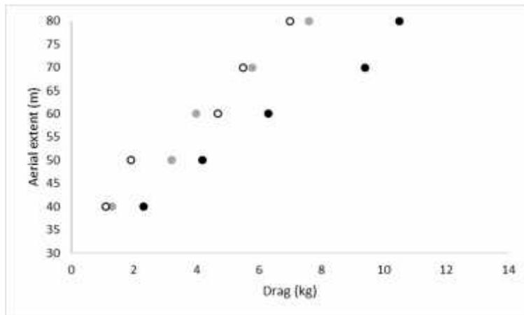
Figure 3. Drag required to achieve tori line aerial extents of 40 – 80 m using three different backbone materials: monofilament (black), Dyneema (open circles), Ashaway albacore braid (light grey) at a deployment height of 7 m.
