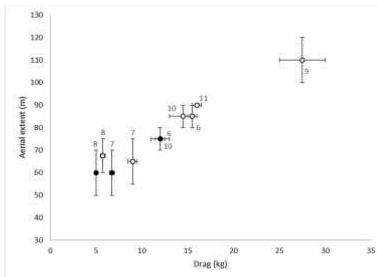
Figure 10. Drag and aerial extent delivered by the tori line designs tested at 6 (black circles) and 7 (open circles) knots on vessel C. Numbers adjacent to points refer to the construction of the tori line (Table 6). The aerial section of all tori lines shown here comprised 70 m of 3-mm diameter Dyneema with single 5-mm orange plastic (T064) streamers placed at 3.5 m intervals. Ranges likely result in part due to swell action during trials.
