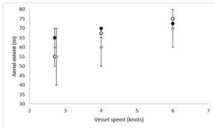
Figure 11. Aerial extent delivered by a tori line tested at deployment heights of 5 m (black circles), 4 m (open circles) and 3 m (grey circles) above the sea surface on vessel C. The aerial section of the tori line comprised 70 m of 3-mm diameter Dyneema with single 5-mm orange plastic (T064) streamers placed at 3.5 m intervals. Ranges likely result from swell action during trial conditions.
