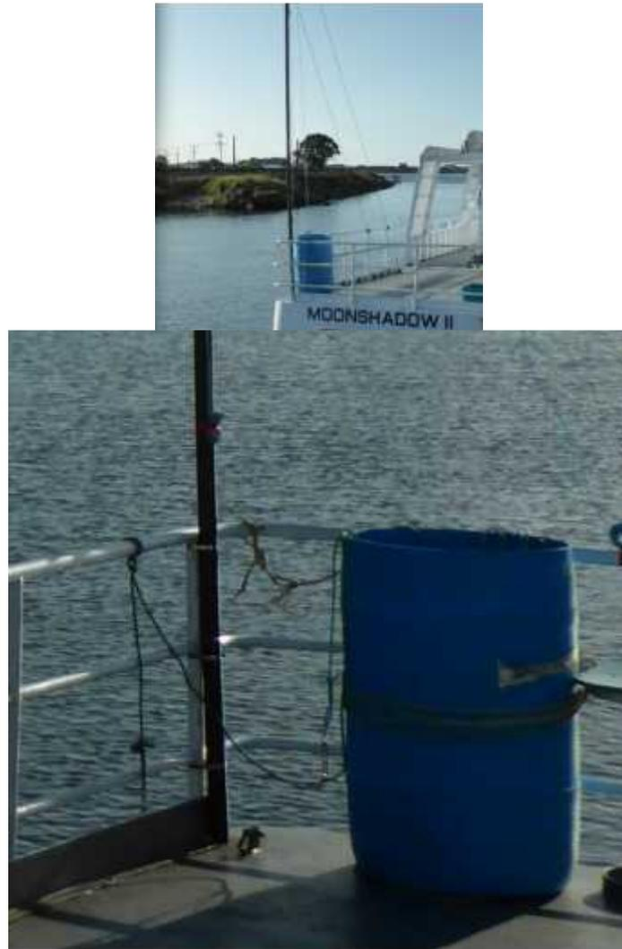
Figure 12. The tori pole attachment, and tori line storage drum, shown in context and close up on.
