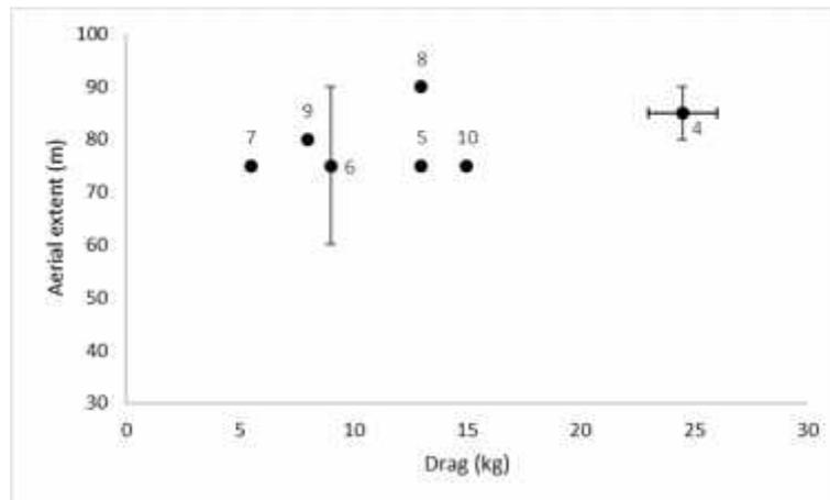
Figure 9. Drag and aerial extent delivered by the tori line designs tested at 7 knots on vessel B. Numbers adjacent to points refer to the construction of the tori line (Table 5). The aerial section of all tori lines shown here comprised 70 m of 3-mm diameter Dyneema with single 5-mm orange plastic (T064) streamers placed at 3.5 m intervals.
