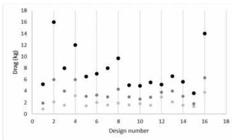
Figure 6. Drag generated from an in-water section of rope with various objects attached, at approximately 2.6 knots (light grey), 4.2 knots (dark grey dots) and 6.5 knots (black dots). Configurations of the in-water section are described in Table 3.
