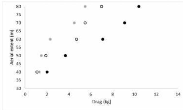
Figure 1. Drag required to achieve tori line aerial extents of 40 – 80 m at deployment heights of 5 m (black), 7 m (open circles) and 9 m (light grey), when 3 mm Dyneema backbone was used with streamers placed every 5 m along the line.
