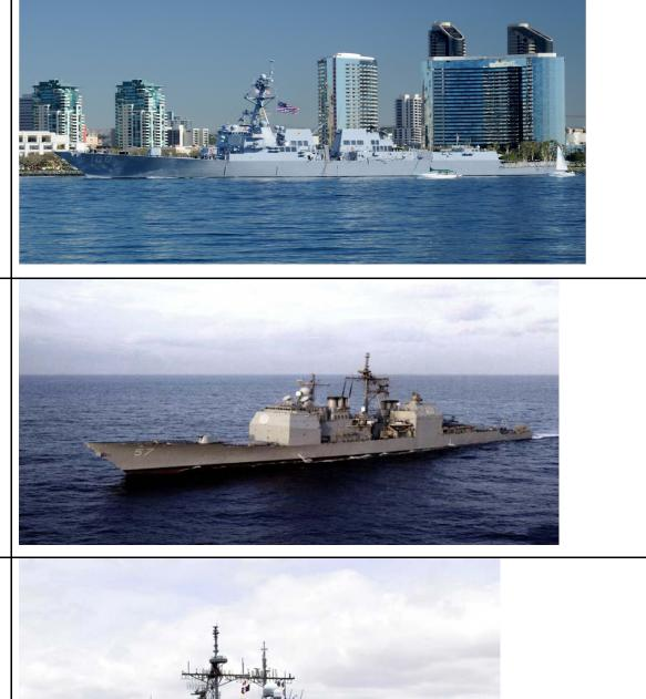
Guided Missile Destroyer Name: USS LASSEN Length: 510 feet Side number: 82 International radio call sign: NLSN Communications: UHF, VHF, and HF
